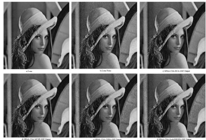
Figure14: a) Lena's Original Image; b) Lena's Noisy Image; c) Proposed Gaussian Filter Output by Applying CSA; d) Proposed Gaussian Filter Output by Employing Approximate Carry-Save Adder (by Applying the Proposed MCSPA Approximate Adder), e) Proposed Gaussian Filter Output by employing Approximate Carry-Save Adder (by Applying Carry Speculative Approximate Adder), f) Proposed Gaussian Filter Output using Approximate Carry-Save Adder (by Applying the Proposed Generic Accuracy Configurable Approximate Adder)
