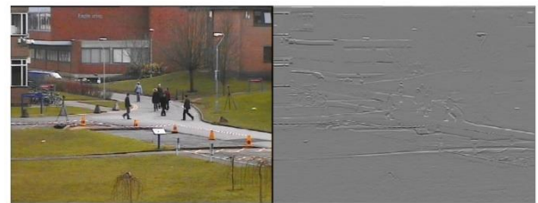
Figure 6. Feature maps extracted from the convolutional layer corresponding to the Figure 2.
